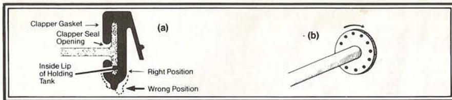
**To Replace Rubber Gasket Seal.** If the bowl does not hold water or there is leakage from the waste holding tank through the flush valve, first check to see if there is some impediment on the outer or inner sealing surfaces of the gasket that needs to be removed. If not, the gasket should be replaced. When replaced, ensure that the gasket is in the proper position inside the holding tank with the sealing surface vertical as shown in diagram A.
