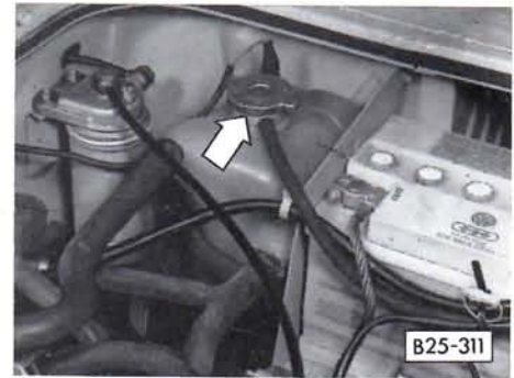
Expansion tank – Diesel engine
