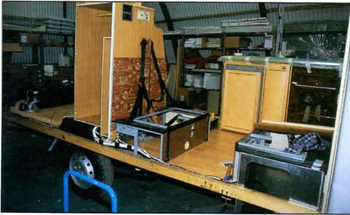
Sandwich construction coachbuilts, like this Palermo, are built 'inside-out' with most of the furniture going in before the side walls and roof being fitted
