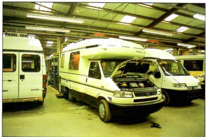
Van conversions and GRP monocoque coachbuilts are built side-by-side
