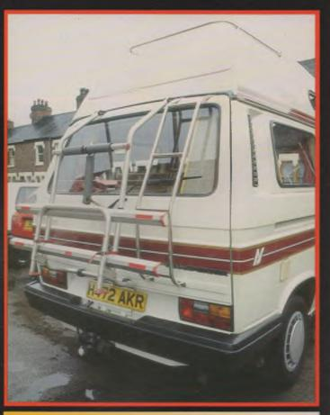
Ladder and roofrack are standard; bicycle carrier and towbar are useful extras making this a comprehensively-equipped leisure vehicle.
