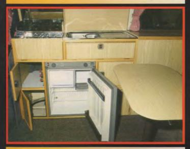
Fridge can operate by gas, mains electricity or the vehicle's battery. Cooker and sink are spotless.
