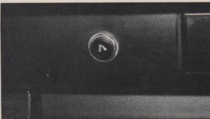
... and cigarette lighter which has 12v DC socket
