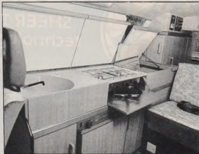
Enamel finish for hob, drainer and sink; melamine-covered splashbacks
