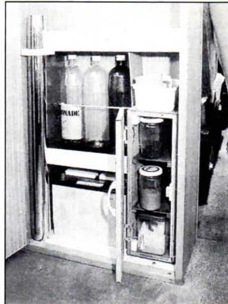
Wardrobe has been converted to hold drinks bottles (note curtain wire restraint), coffee jars etc. Table leg stows in spring clip (left) and spare battery fits in the bottom.
