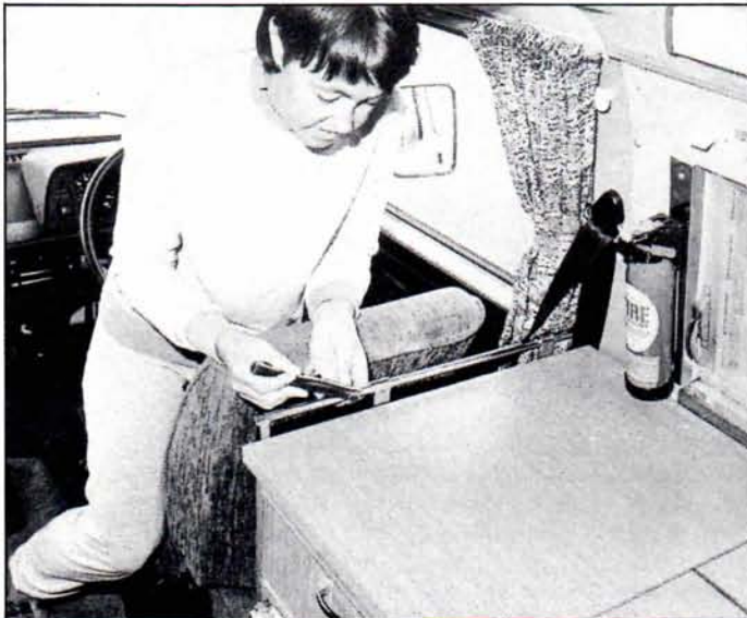
To prevent sink top sliding along the chrome bar it is necessary to fit a piece of plastic tube (split lengthways) when van is being driven. Above fire extinguisher is 12 volt plug and water tank gauge.
