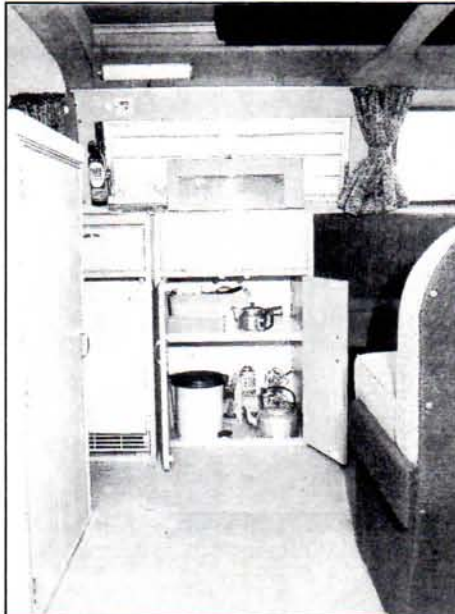
View through side door shows storage cupboard under cooker, 2-way fridge with sink above and wardrobe on left which has been converted to provide extra storage space.
