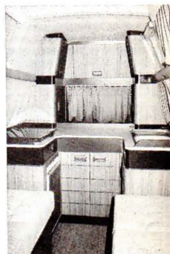
Kitchen and storage units occupy the rear of the Holdsworth VW Variety in a novel layout. Rounded corners bring a look of up-to-the-minute style and quality to the furniture.
