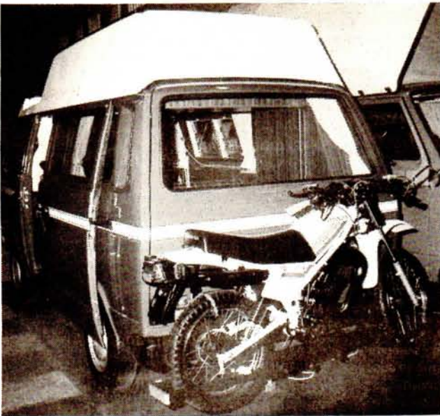
A Motorhomes International VW Motorsleeper with rear-mounted motor-cycle. With its 50/50 weight distribution the new VW can take such a load with little effect on handling.
