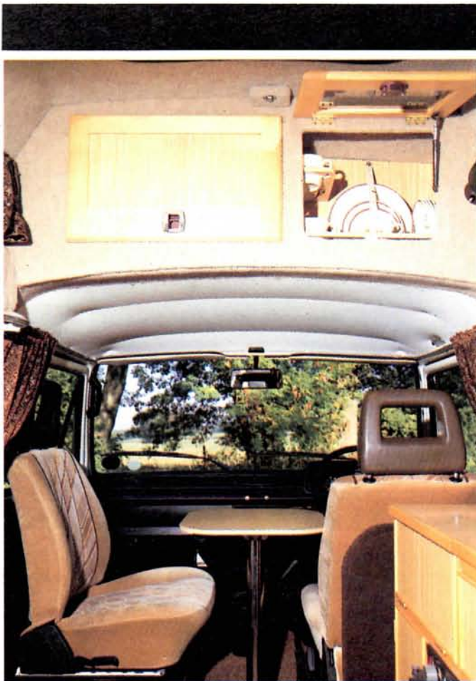
Swivelling cab passenger seat and 21-piece crockery set are standard; the cab table is optional
