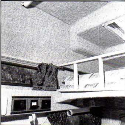
Electrical fittings include a 12v water gauge and a mains socket
