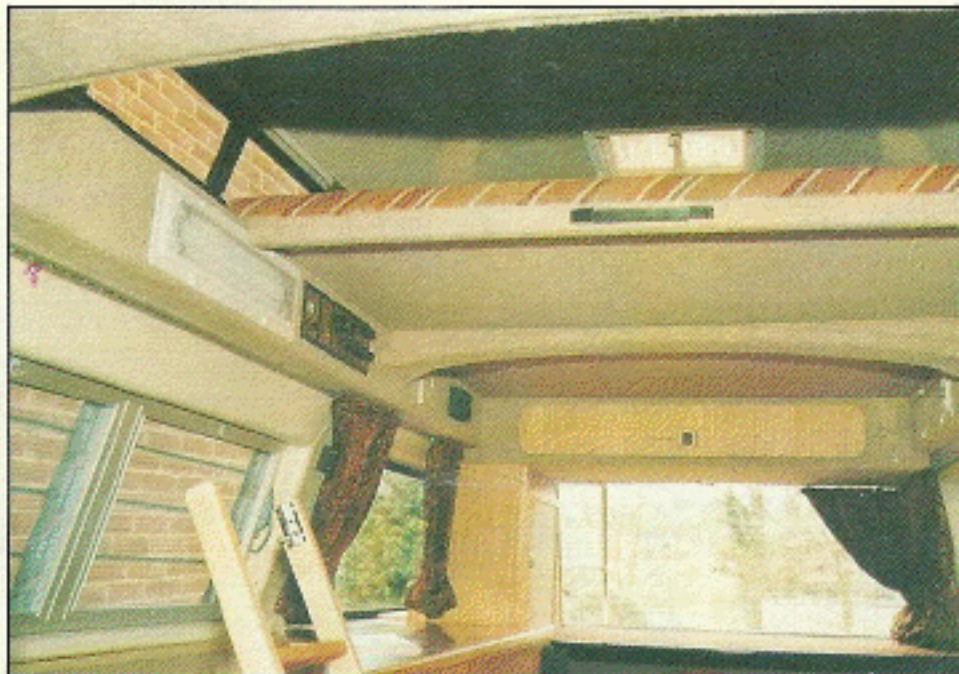
Upper bed pulls forward into position from above rear roof bow. Luggage-restraining ladder is used to climb up via kitchen work-surfaces. Ladder has no anchorage points.
