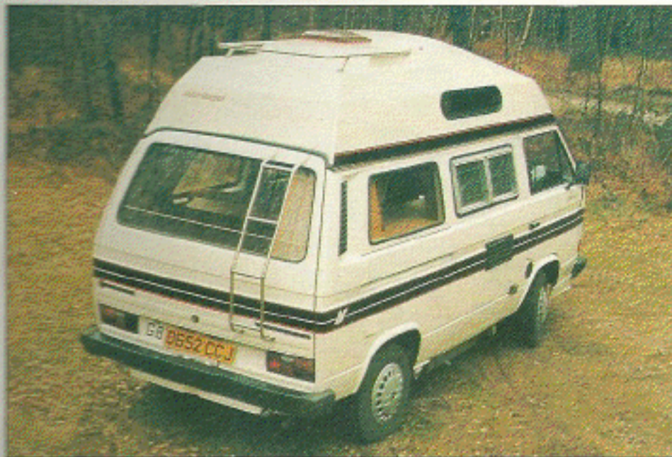
Roofrack is moulded into roof, does not jut up into airflow. Exterior coachlines have been restyled on latest models, and louvred window replaced with sliding type.
