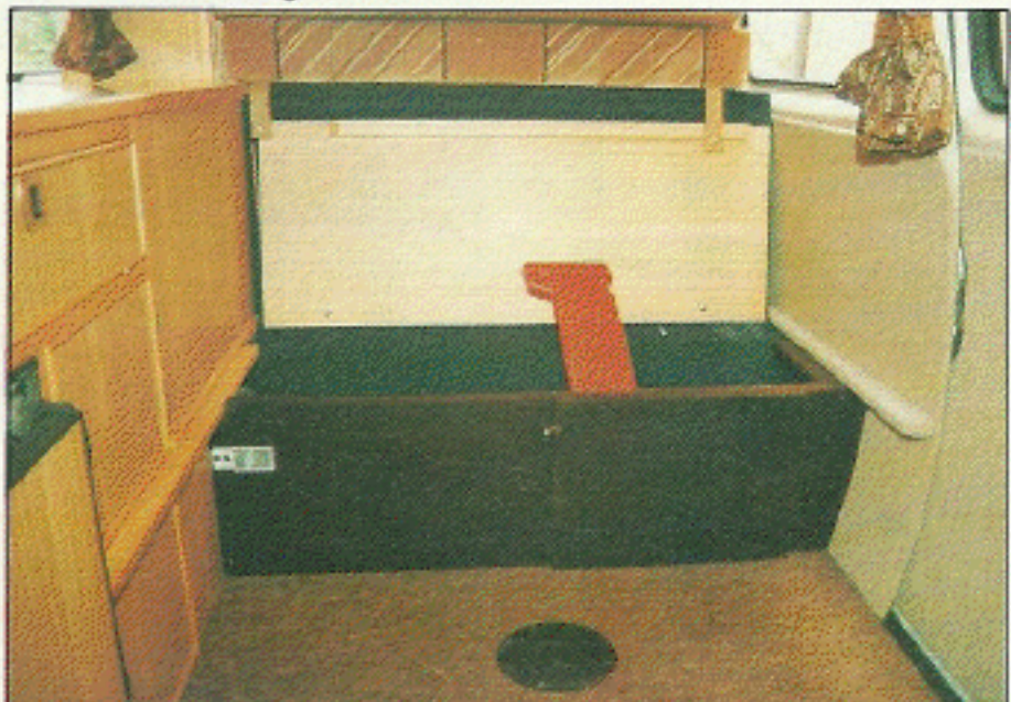
Extra storage is provided beneath settee forward of engine deck. Flap on front of settee base folds out for bed support. Note mains hookup ELCB controls easily accessible beneath settee.
