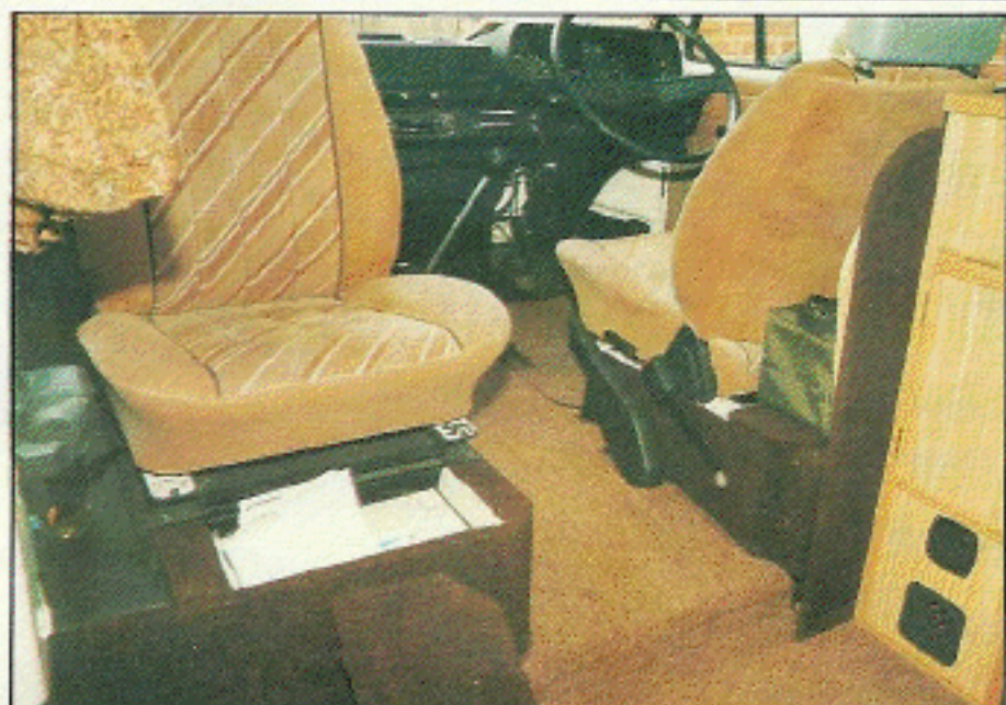
Passenger seat could be moved to hide small storage compartment below. Dining table stored behind driver's seat, yet left room for assistant editor's camera bag.
