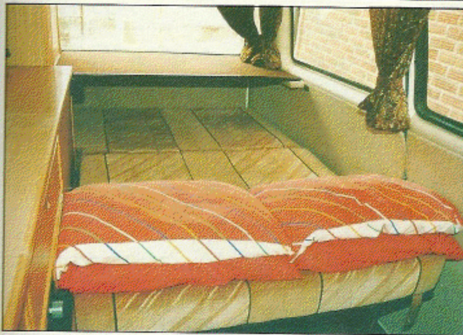
Parcel shelf can be left in position with pillows at forward end, but bottoms of curtains tend to hang away from side door. Fluorescent light and Propex control can be reached from bed.
