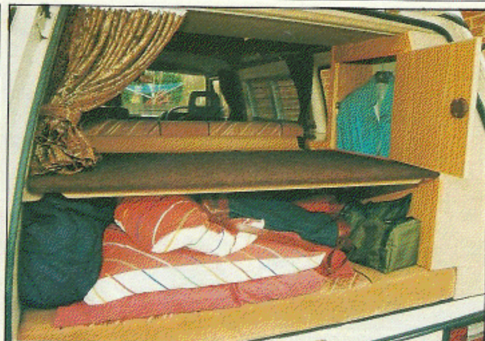
With tailgate closed, parcel shelf conceals shopping or other goods. Wardrobe door opens through 180 degrees to allow access from inside or out.
