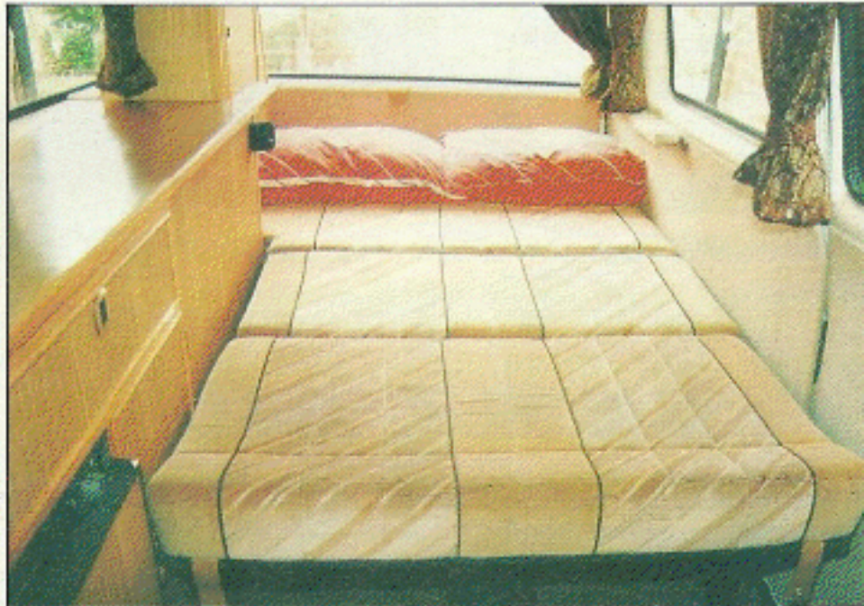
Lower bed prohibits use of one kitchen cupboard, but fridge and Porta Potti/gas compartment are still accessible. With pillows at wider rear end, storage must be found for parcel shelf.
