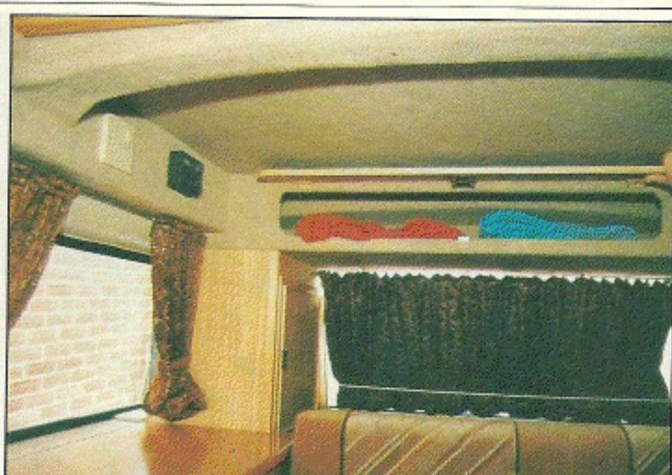
Shallow locker beneath upper bed would benefit from supporting stay on door. Door remains well clear of heads as it is sensibly top hinged.
