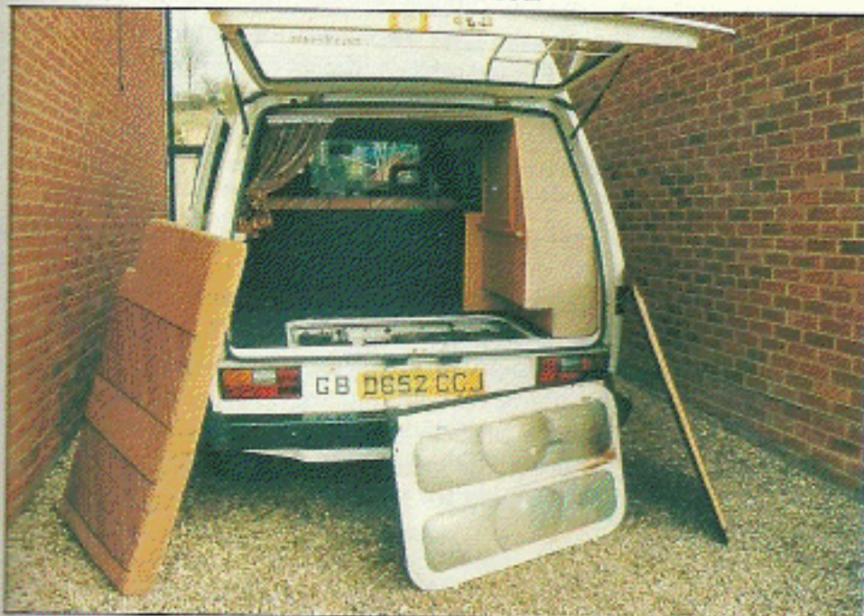
Parcel shelf, rear mattress section and engine cover all lift out easily for engine servicing. Daily checks are carried out through hinged number plate.
