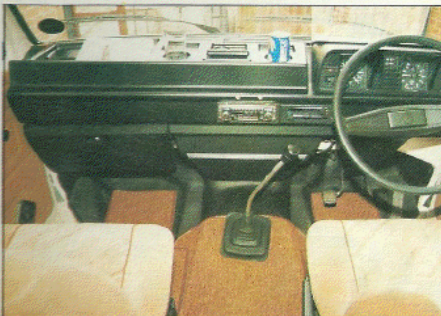
Neither gear lever nor handbrake obstruct walk-through from cab. Footwell mats match caravan carpet and are easily removable for cleaning. The Onex dashboard fitting provided some additional cab storage.
