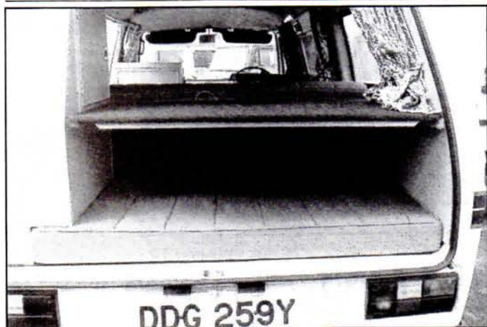
The 'boot' at the rear end. Shelf hides shopping from the inquisitive. Shelf and cushion can be quickly removed for access to engine below. Oil and water points are behind number plate.
