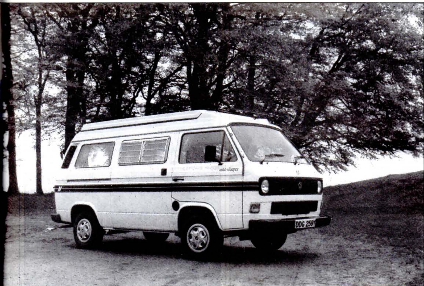
△ VT20. Auto-Sleepers' low-line rising roof keeps overall height just below 7ft. Like Renault, VW has small roof rack over cab and prominent side striping bearing A-S motif. But note the Volks's superior wheel trims.
