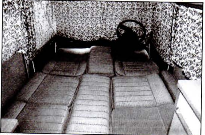
RV50. Using backrests and extra cushions to make up the 5ft 5in wide king size bed. Front centre cushions may appear to stick up a bit — but that's where feet go and it's not uncomfortable.
