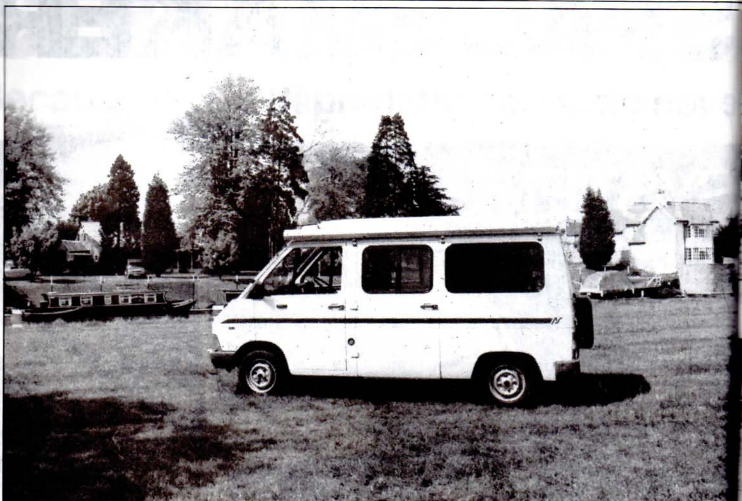
△ RV50. Short wheelbase version of front wheel drive Renault Traffic is car-like in size, parkability and ease of driving. Spare wheel mounted on rear door is accessible and clean but length is increased marginally.
