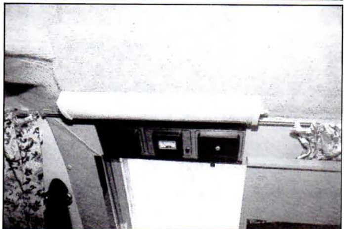
VT20. Above kitchen unit is flyscreened louvred window; above that new control panel incorporating fuses, 12 volt socket, water level gauge and master switches for interior lights and water pump.
