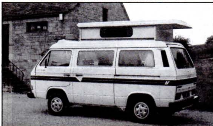
▽ VT20. The rising roof was effortless to raise but upper bed had to be shunted to and fro when fastening side panels and it was necessary to stand on seat to reach rear bolts. Centre locking desirable here.
