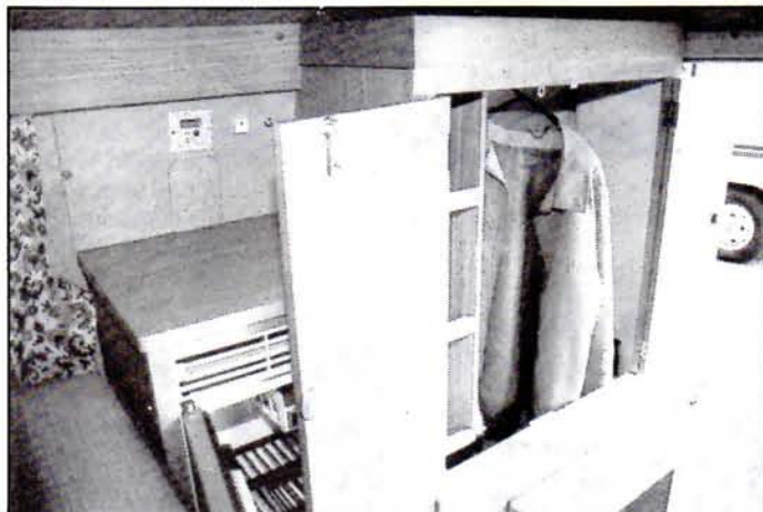
RV50. Opposite kitchen is wardrobe with incorporated lipped shelf unit and flat top, also with lip. Forward of that is 'frig and another flat top. Above is fuse panel, water level gauge and 12 volt socket.
