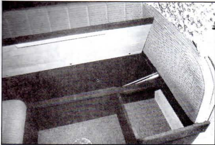
VT20. Storage beneath rear seats. Note carpet lining throughout. Square locker on right of photograph will hold small chemical closet or walls will concertina away for extra floor space.
