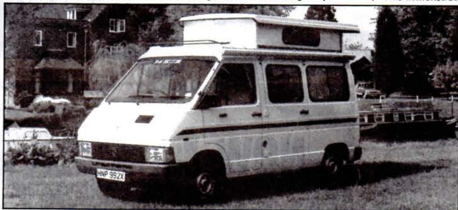
△ RV50. Short wheelbase version of front wheel drive Renault Traffic is car-like in size, parkability and ease of driving. Spare wheel mounted on rear door is accessible and clean but length is increased marginally.
