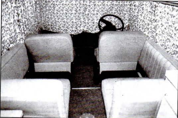
RV50. Four forward-facing seats for travelling. Settee backrests on side walls make arm-rests, offside one hides table stowage. Carpet is flecked and doesn't show marks. Note 'modesty skirts' on backs of front seats.
