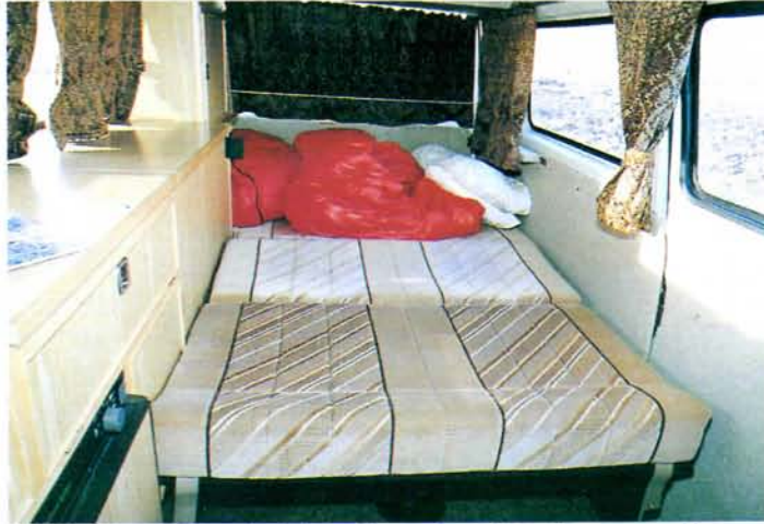
This is how the lower double bed is made up from the seats and back cushion.
