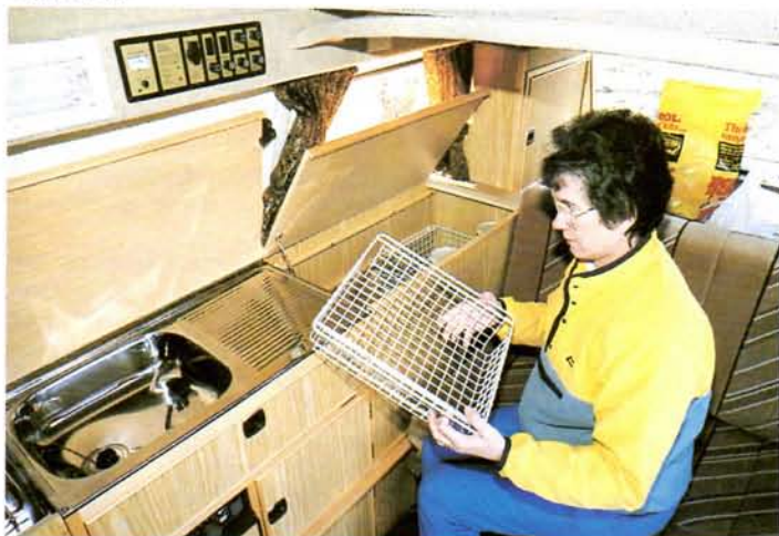
Wire baskets fit into lid closed storage cupboard. Sink is stainless steel with powered water supply.
