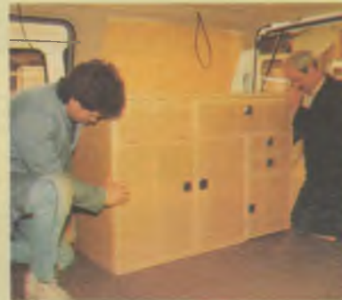
The kitchen is assembled before being mounted in a Ford Frisky.
