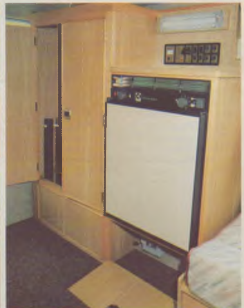
High level fridge/freezer with control panel above.
