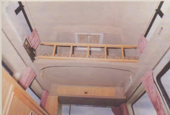
Dual purpose wooden ladder: keeps luggage in place and aids access to upper double bed.
