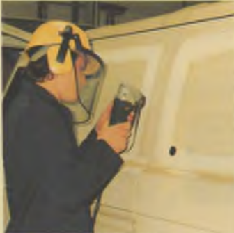
An electric nibbler is used to cut the apertures for windows.
