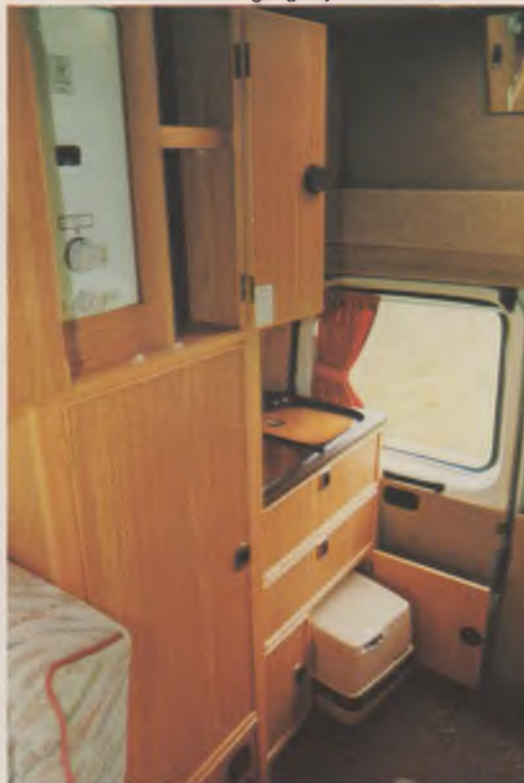
Water heater above wardrobe, sink unit beyond.
