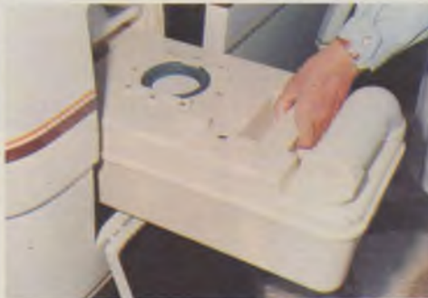
Easy removal of Cassette waste unit — from the exterior.
