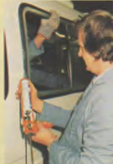
Two operators fit and seal the windows
