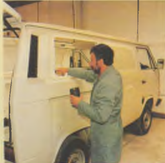
Window apertures and other cut edges are treated to prevent rust.
