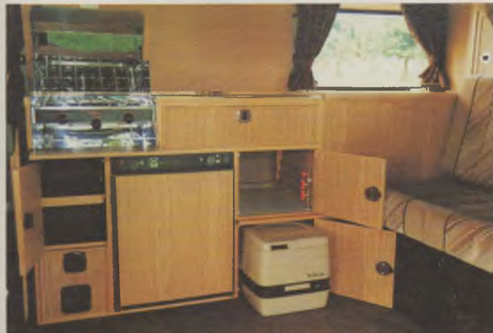
Well appointed kitchen. Outlets for optional blown air heater are shown lower left.
