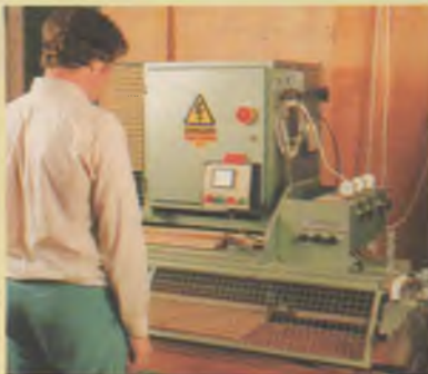
Hardwood edges for worktops and furniture are now bonded by microwave.
