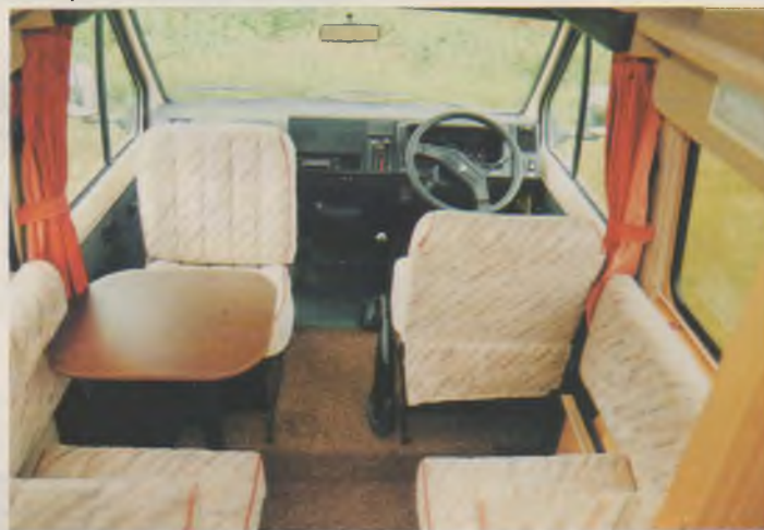
Passenger seat reverses to face single dinette, optional for driver's.
