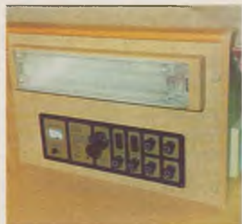
Consideration for the user: in addition to water gauge and switches the control panel contains accessible and identifiable fuses.
