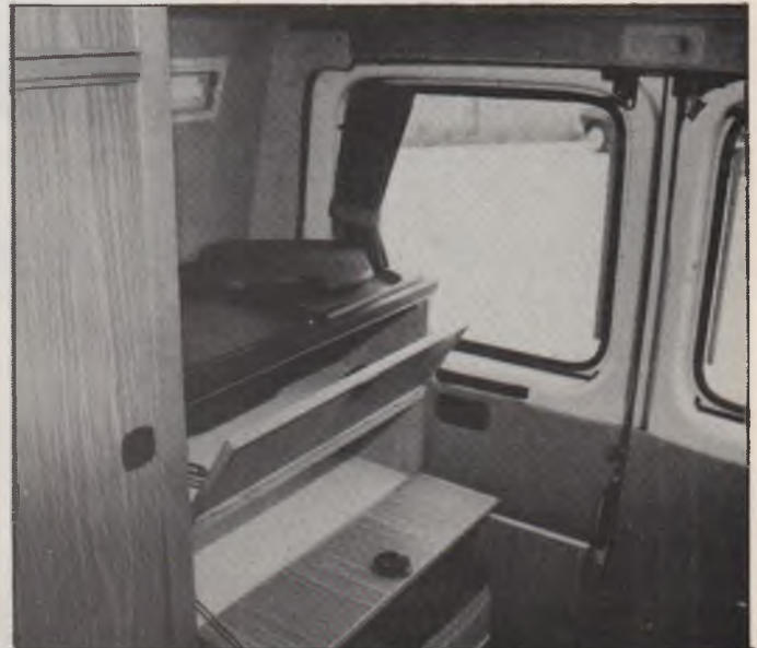
Sink unit with h & c water storage and chemical toilet below
