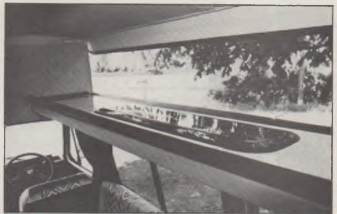
Roof side panel can be folded down to provide 'Grandstand' viewing
