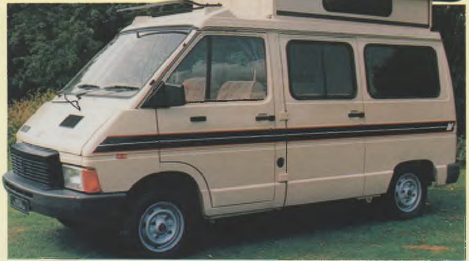
Solid type construction, insulated elevating roof in raised position
