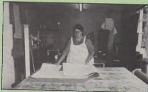
Carpet and trimming shapes are cut from template guides in a separate workshop
