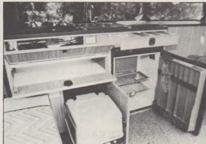
Cooker/Sink/Fridge unit with chemical toilet below and seat on the left
