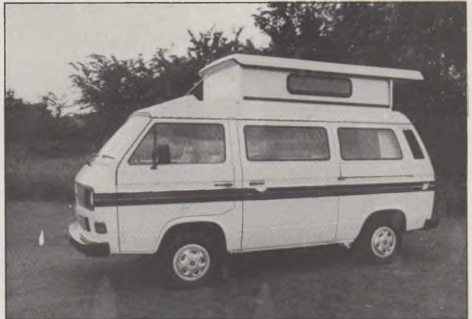
Easy to operate, insulated roof, in raised position
