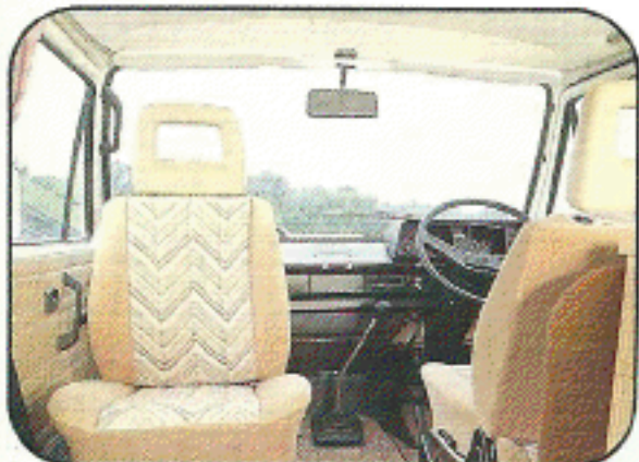
Passenger seat swivels for maximum use of space.
